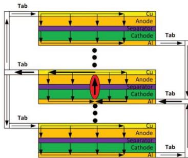
**Figure 1** Current flow path in the internal shorting process
