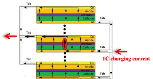
**Figure 8 Current flow path in the internal shorting process with charging for large shorting resistance (2 Ω)**
