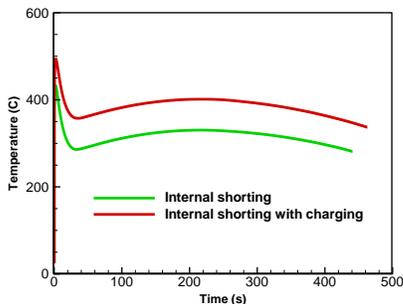
**Figure 5 Temperature responses at shorted location (10 mΩ)**
