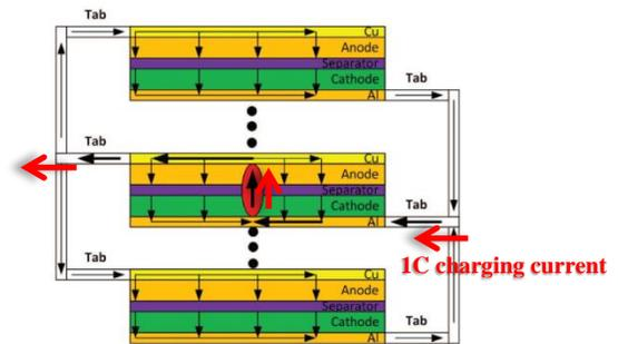
**Figure 4** Current flow path in the internal shorting process with charging for small shorting resistance (10 mΩ)
