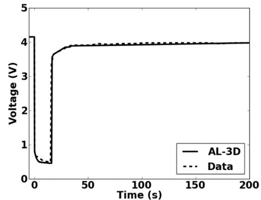
**Figure 2. Simulated and experimental cell voltage during external short.**
