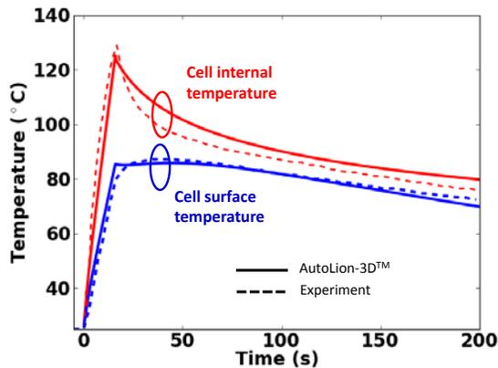
**Figure 4. Simulated and experimental temperature during external short. Red curves represent cell-internal temperature at center of cell, blue curves represent surface temperature; dashed lines represent data and solid lines are simulation.**
