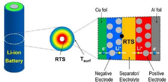
**Figure 1. Diagram of 18650 cell embedded with reaction temperature sensor (RTS), along with surface-mounted temperature probe [3].**
