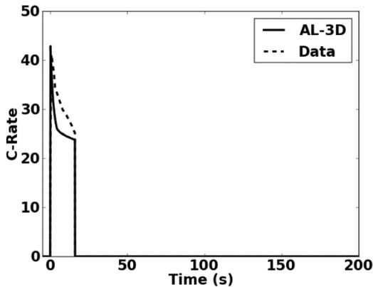
**Figure 3. Simulated and experimental cell current (C-rate) during external short.**
