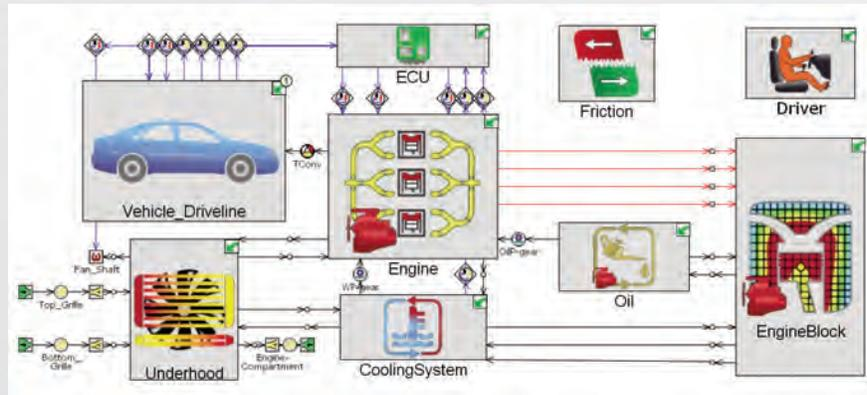
Similarly, an entire vehicle model with a dynamic pulsating engine shown below executes at 0.7-0.8 times real time and therefore can be used for HiL applications
