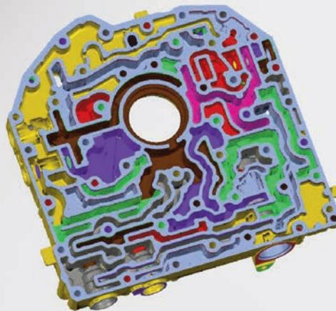
Discretization of a 3D CAD model into a GT-SUITE model
